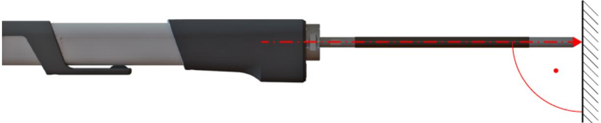
2. Press the sensor against the object with sufficient and consistent pressure.
