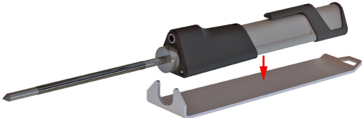
2. Screw the required waveguide in the sensor's ultrasonic transducer.
