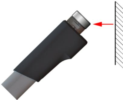
3. Carefully push the protective pad sideways on the magnetic waveguide.
