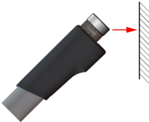
4. Carefully tilt the sensor on the point of measurement until the magnetic waveguide rests on the point of measurement with its complete surface.
